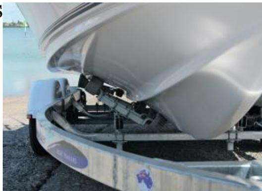
The Haines Signature 575RF hull features wide, reversed chines and prominent strakes. The kicker step at the bow is said to reduce 'sneezing' spray forward.
