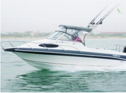
The deep V at the front and a variable deadrise means that rough conditions can be handled with ease.
