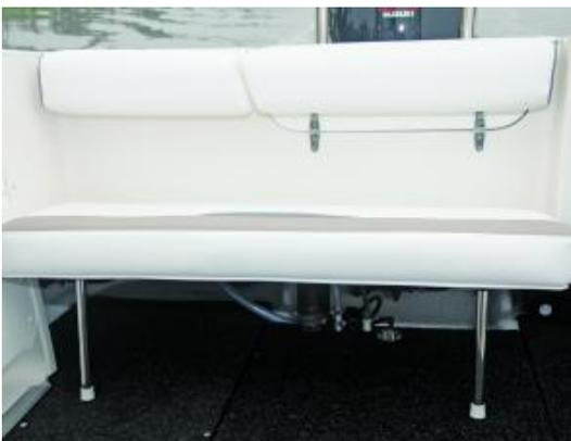
Fold-down rear bench seat also flips up for access to the batteries.
